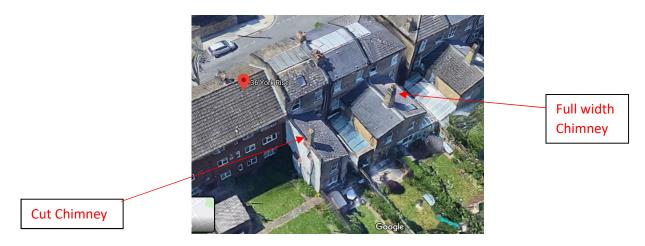
Reduction of width of chimney stack resulted in a slender brick structure with reduced resistance against the overturning, condition of the brickwork also deteriorated over the time. Considering these facts, I recommend to remove the chimney stack completely above the roof to eliminate the associated risk of structure failure.
