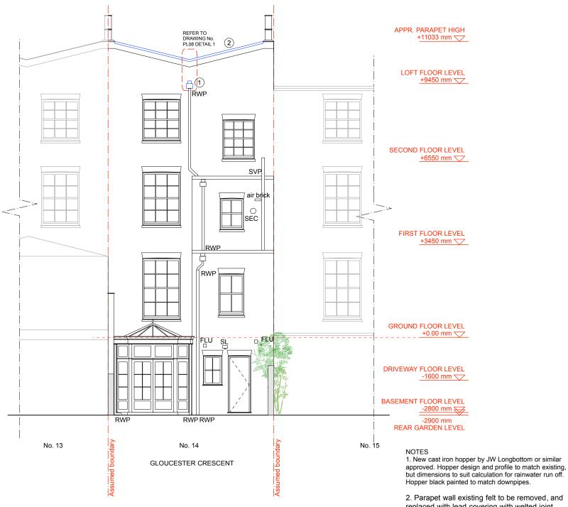
2. Parapet wall existing felt to be removed, and replaced with lead covering with welted joint. Dress lead over parapet wall 75mm and neatly fold under. Secure lead with copper or stainless steel clip as per Lead Sheet Association or
