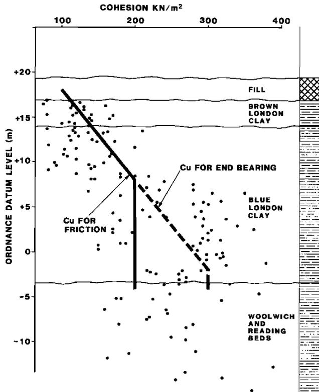
Fig 6. Cohesion values determined by site investigation
