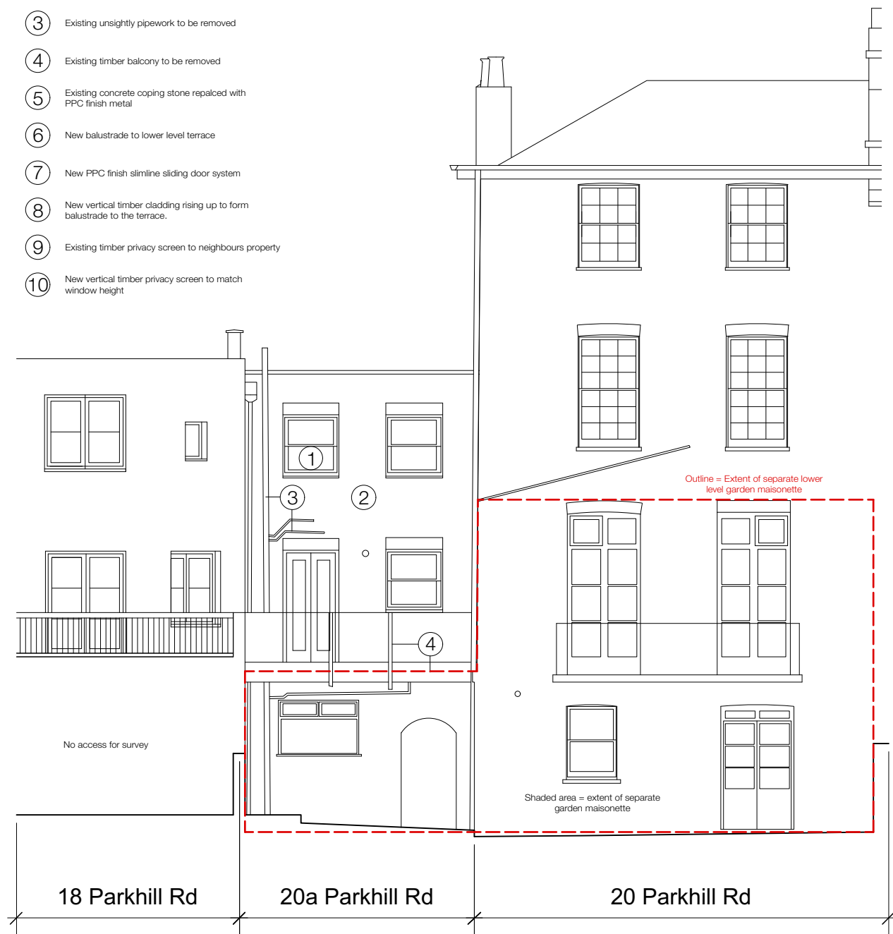
Existing Rear Elevation
