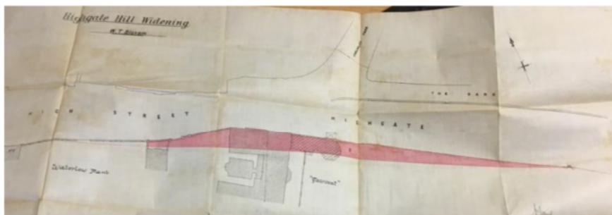
Extent of Fairseat Demolition early 1900s
