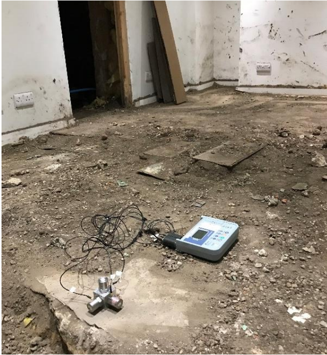
Figure 3 Photograph showing vibration measurement location
