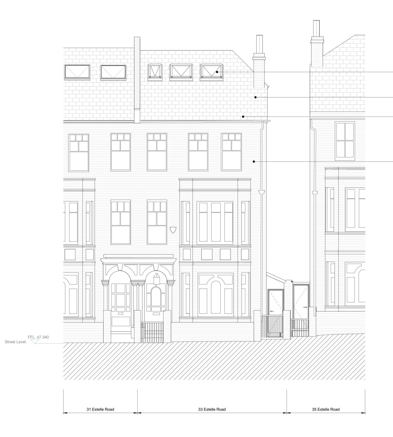
New double glazed opening rooflights to loft extension
