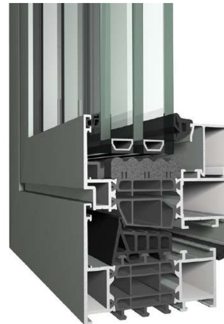
Raynaers Masterline 8 System system datasheet and cross profile. The base and side profiles will be partially concealed by the surrounding cladding to achieve a reduced sight-lines.
