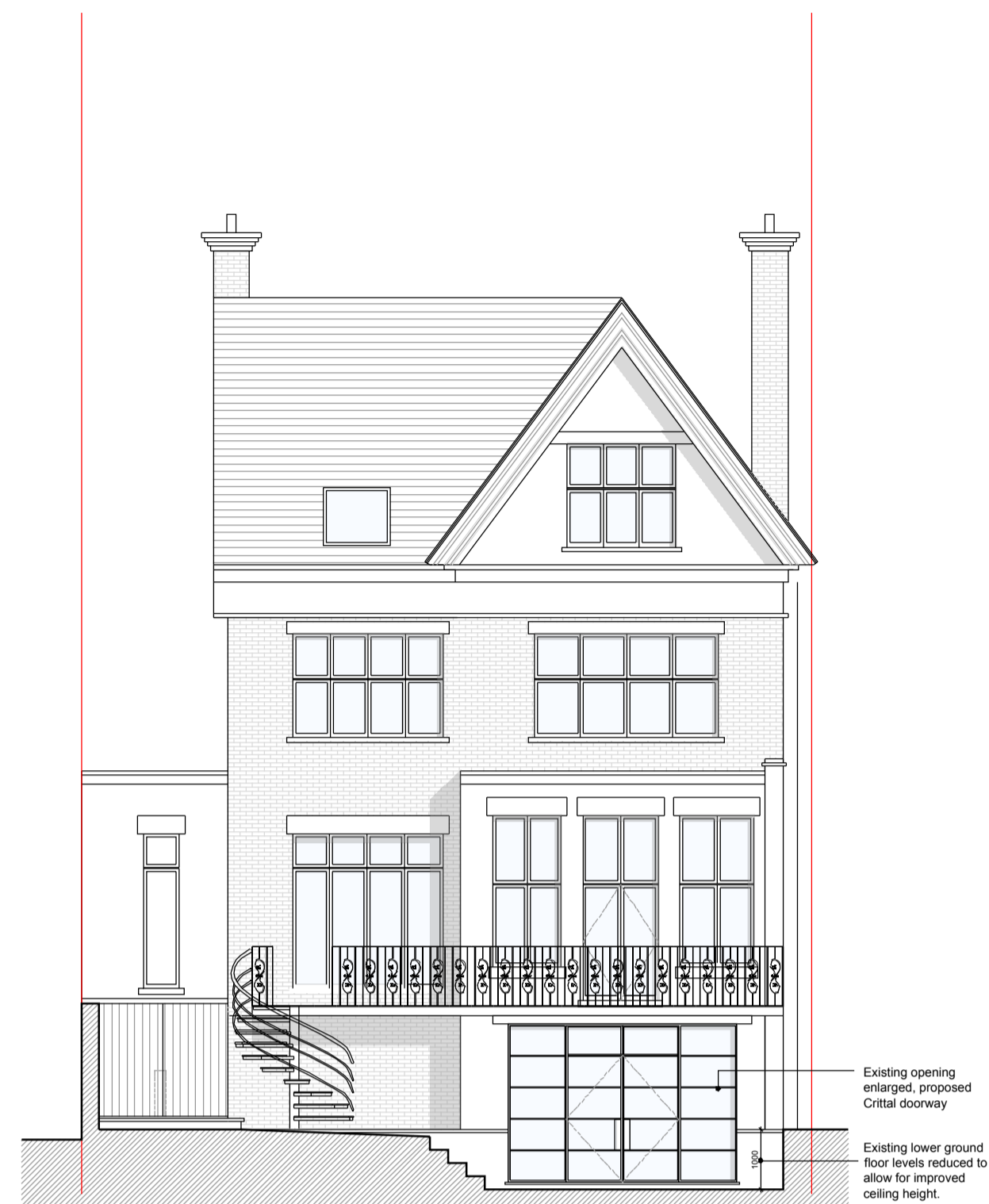
EXISTING REAR ELEVATION
