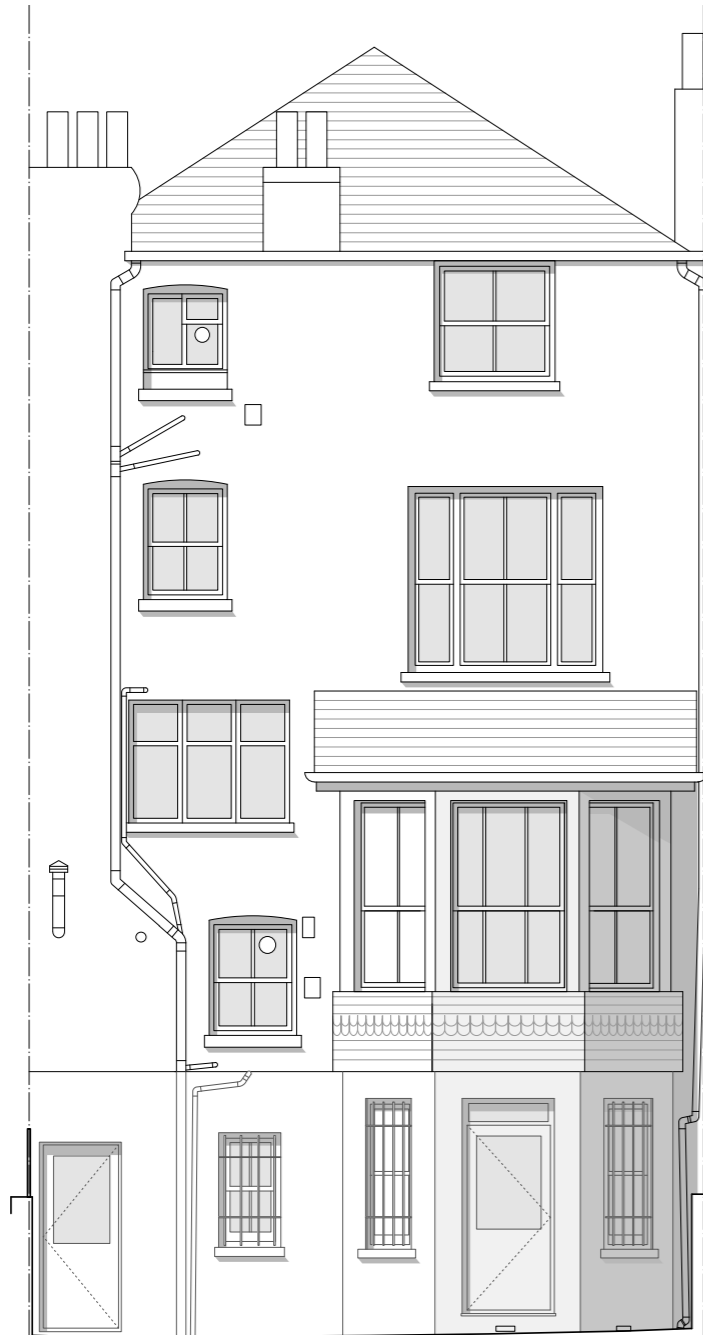
▲ Fig 12. Existing rear elevation. Modern PVC doors at lower ground level clash with a language of painted timber sash and casement windows.
