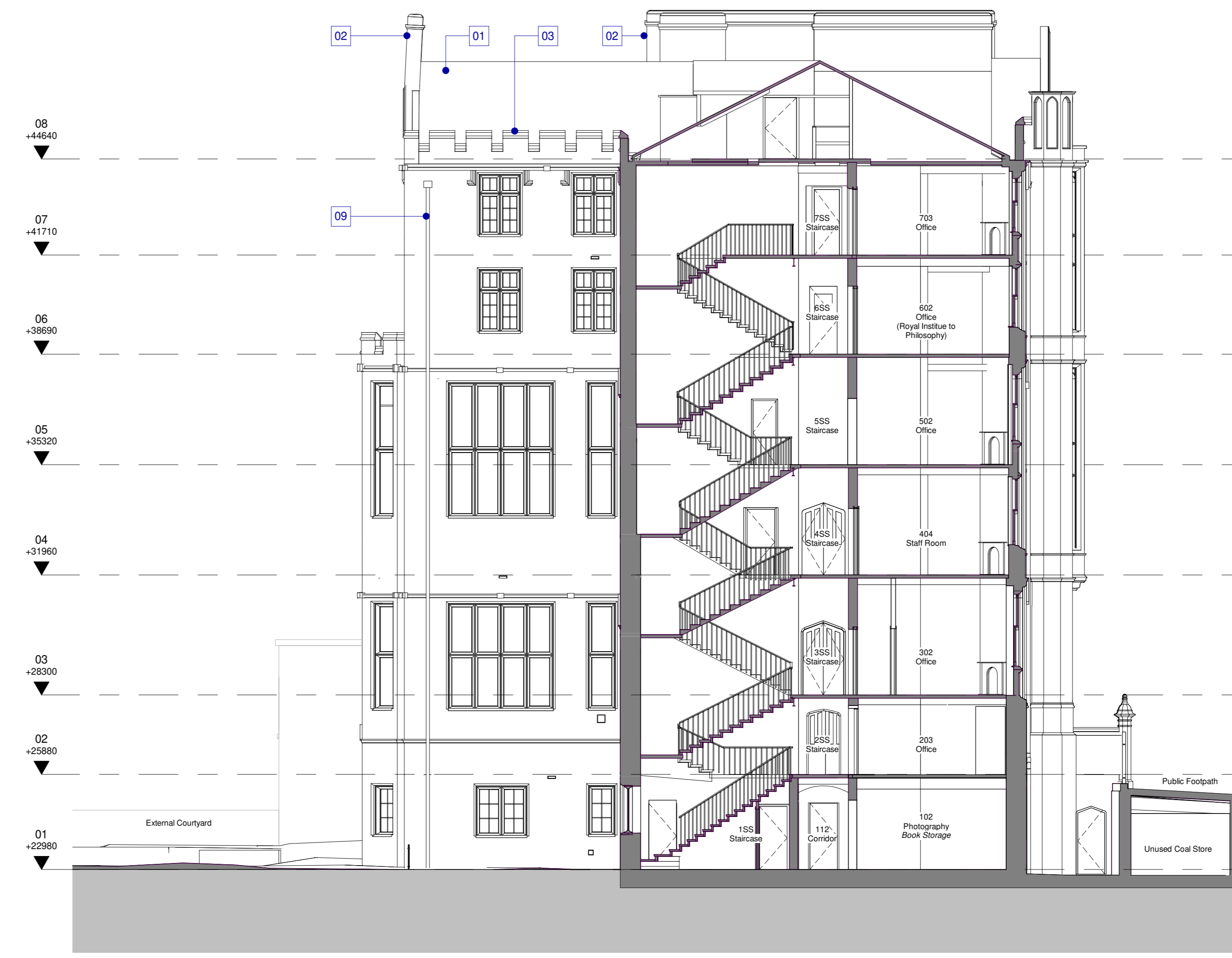
GA Elevation - Central Wing A 1 : 100
