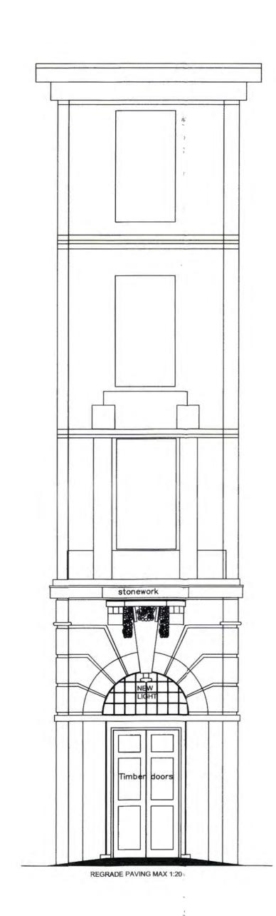
**EXTERNAL WORKS:** Install new task lighting proposed above ATM, night safe, entrance and letterplate as per M&E specification. Regrade footpath to level threshold to comply, allow for all making good as necessary.
