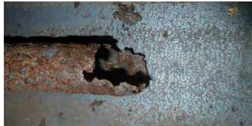
Corroded pipe found on site
