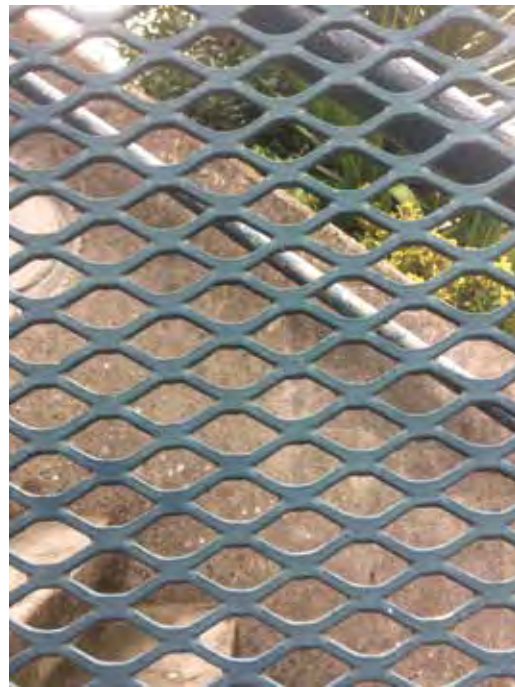
Expanded metal - blue protective coating
