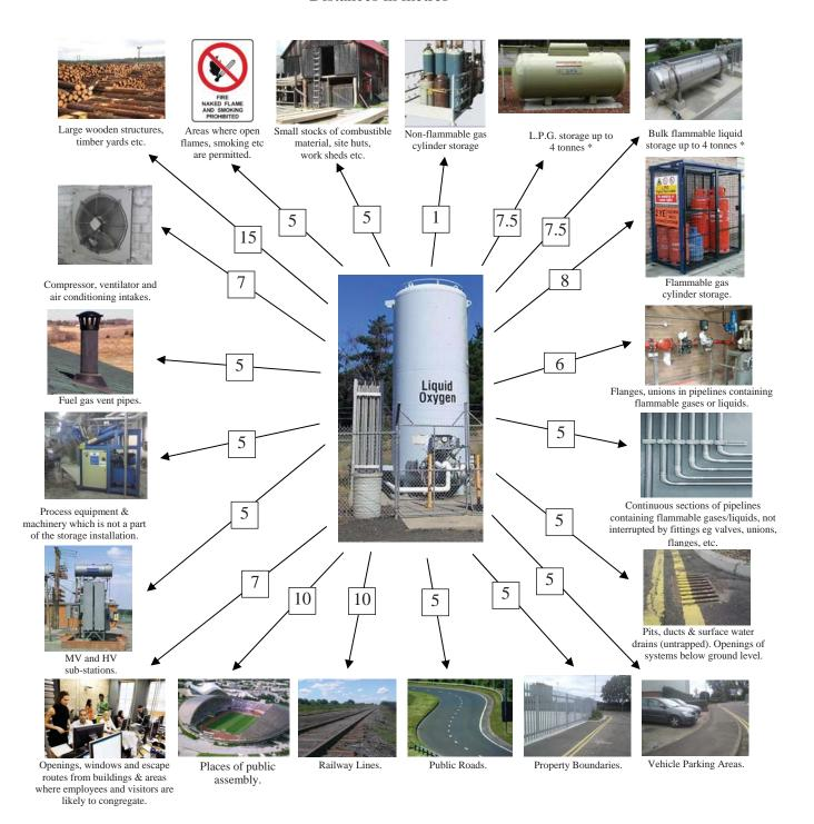
NOTE: Assumed maximum oxygen liquid phase pipework diameter DN 40 (1½" nominal bore) and flammable gas / liquid pipe up to DN25 (1" nominal bore).
