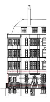
As part of the works, the client wishes to replace all existing windows with inkeeping/heritage windows that improve the condition and thermal properties, and remove the need for secondary glazing.
