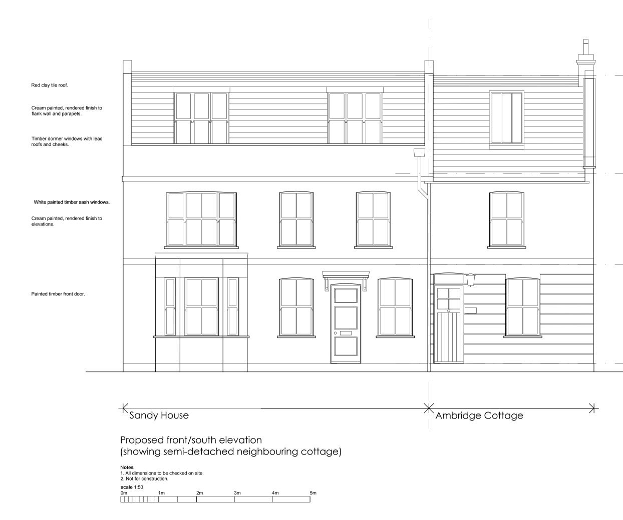
Existing flank wall and chimney raised to suit new roof profile. White painted, rendered finish. Clay chimney pots re-used with all details as existing.
