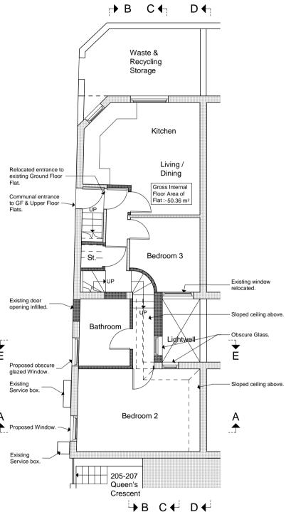
**Proposed Ground Floor** / Upper Ground Floor Plan
