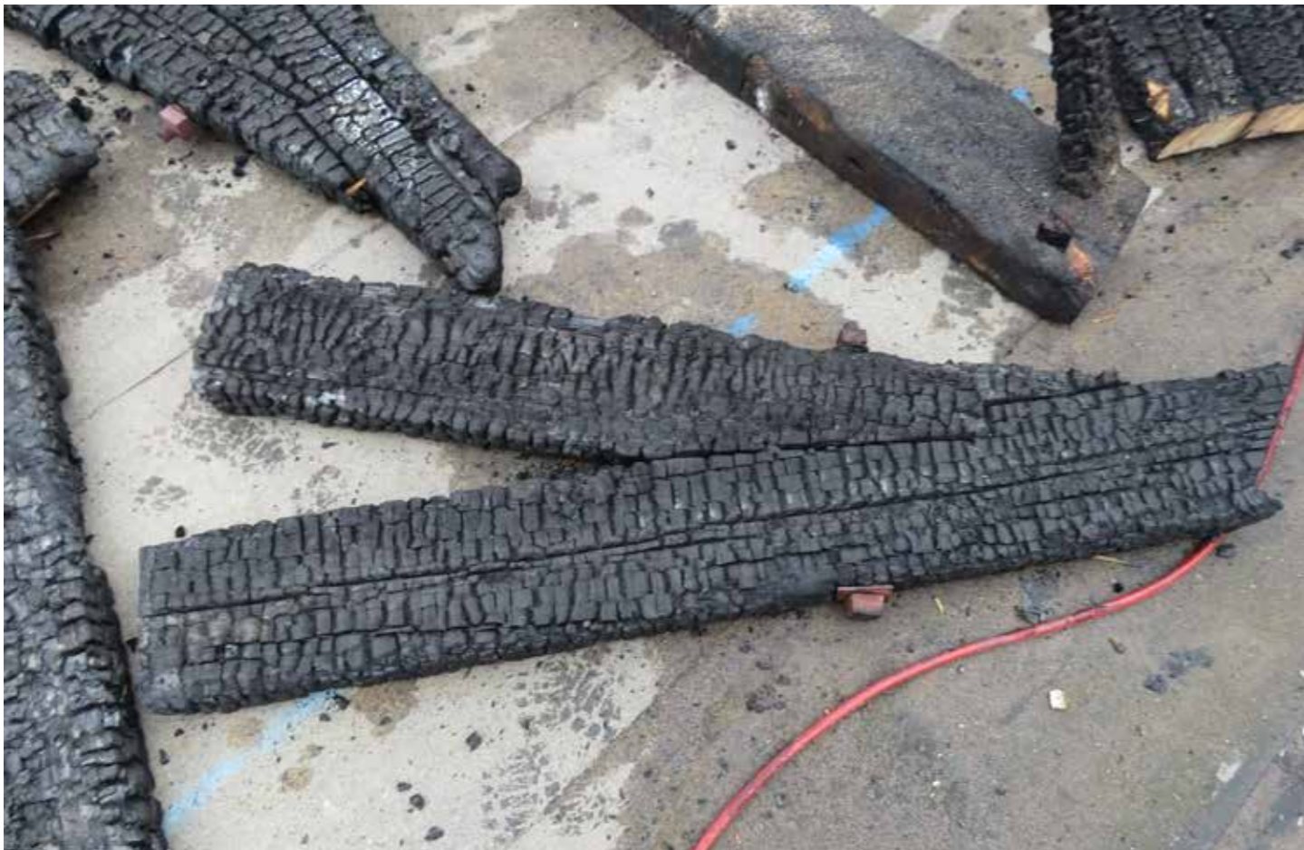
Figure 158: Sample #24 - Bolted metal brace (T4) connecting tie beam (T1) to principal rafters (T3) sample taken (2020) © SLHA
