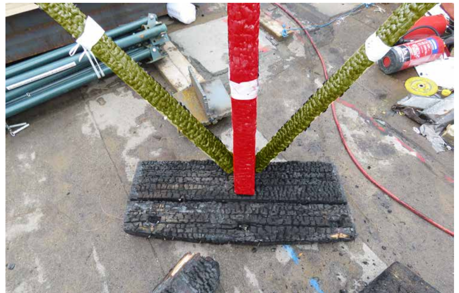
Figure 46: Sample #2 - Junction between main support post (A) with braces (G) and upper rafter plate (E) (2020) © SLHA
