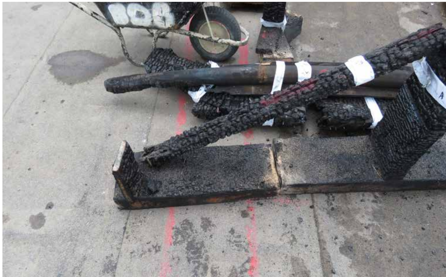
Figure 51: Sample #4- Junction between main support post (A) and braces (G) on inner lower stud wall plate (D1) (2020) © SLHA
