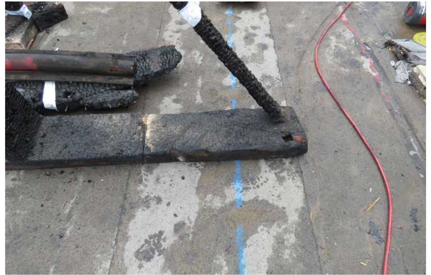
Figure 86: Sample #13 - End of inner lower stud wall plate (D1) with supporting braces (G) (2020) © SLHA
