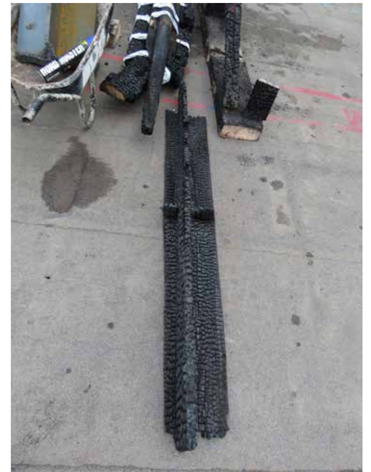
Figure 64: Sample #5 - Wall studs and ties (B) with wall boarding (H) (2020) © SLHA
