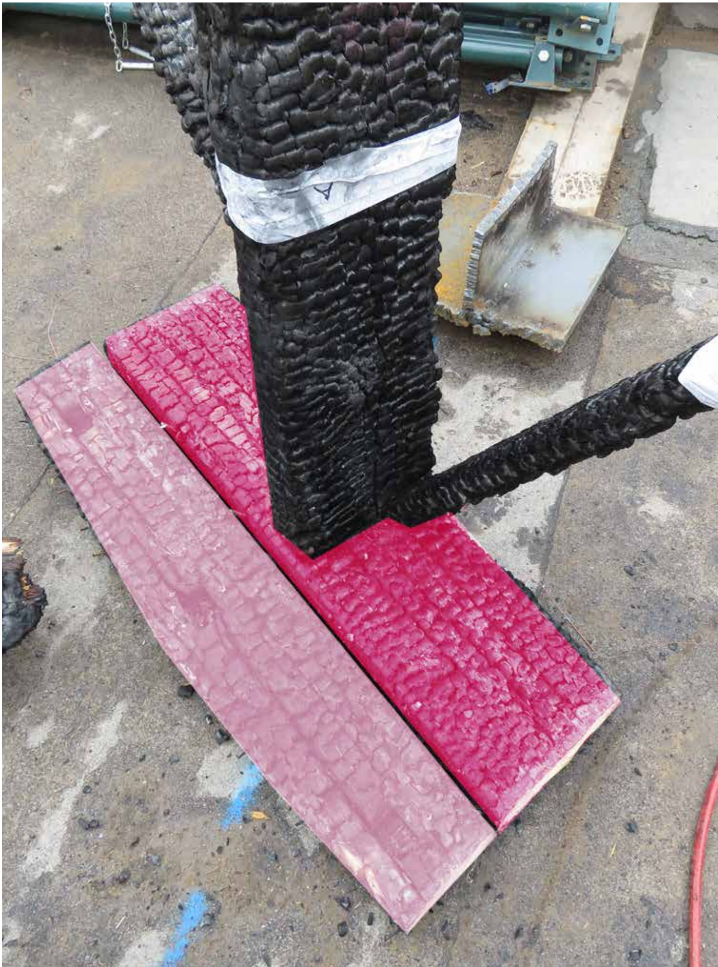
Figure 93 Sample #15 - Upper rafter plates (E) sample taken with the main support post (A) and supporting braces (G) (2020) © SLHA
