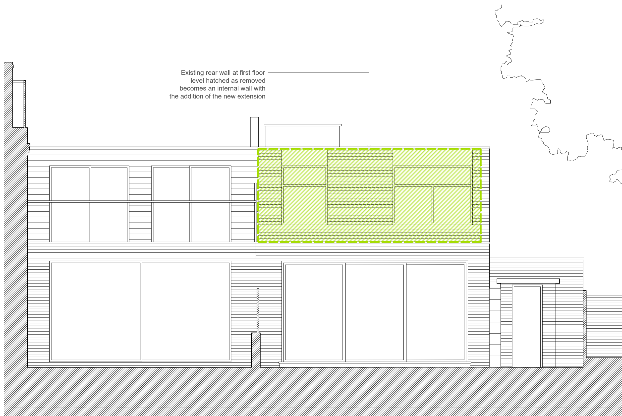
836/40 Existing Rear Elevation
