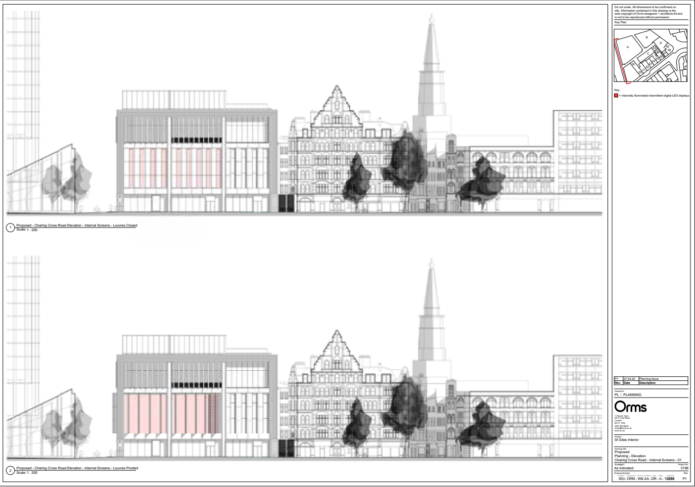
Figure 3.8 Proposed Charing Cross Road digital screens with the louvres pivoted. Drawing not to scale, by ORMS.
