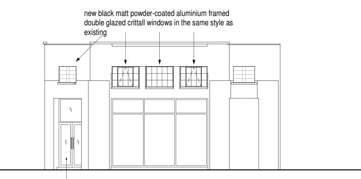
New entrance door & panel above (to replace old ones) to be powder coated aluminium framed double glazed - colour and style to match existing
