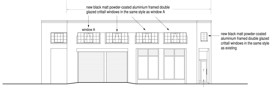
new powder coated aluminium framed double glazed door to replace previous old one - colour and style to match existing
