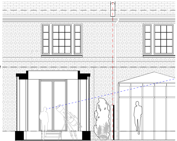
Proposed section through the conservatory - overlooking is prevented by the lowered floor level, the existing boundary fence and new planting.
