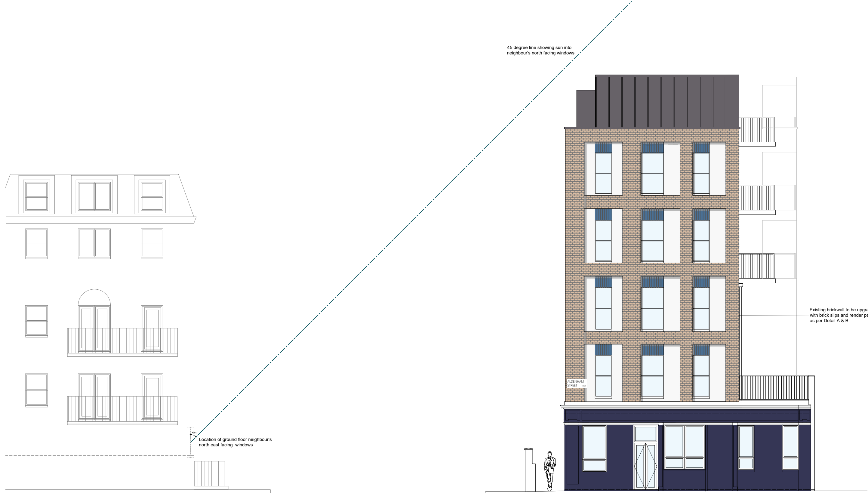
PROPOSED SIDE ELEVATION facing Aldenham Street Scale 1/100
