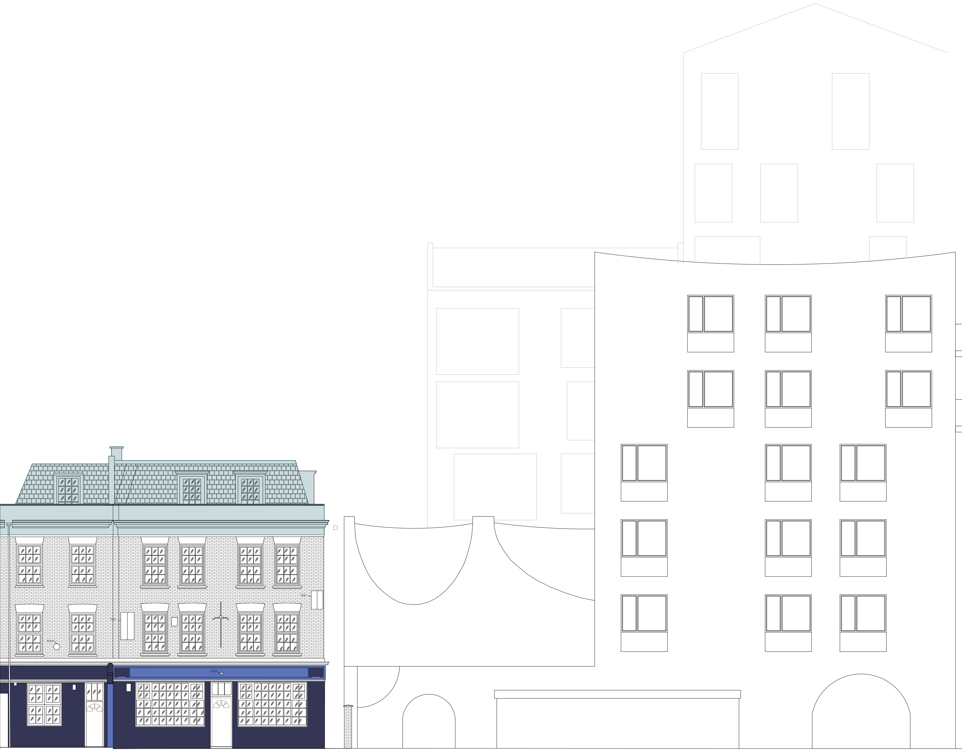
Existing FRONT ELEVATION facing Chalton Street Demolition highlighted in Green Scale 1/100
