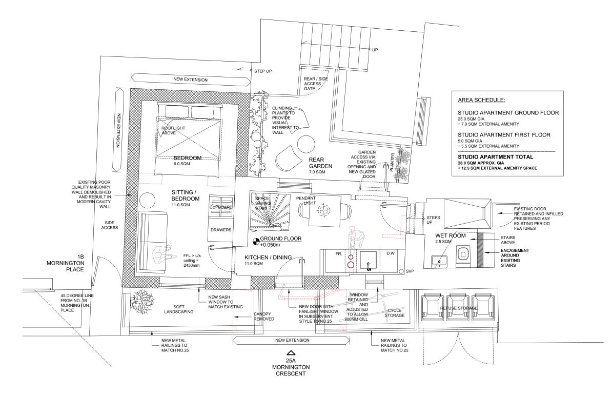
PROPOSED GROUND FLOOR PLAN SCALE 1:50
