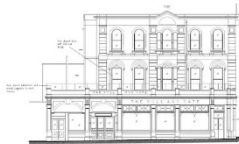
FRONT ELEVATION A-A Concept elevation drawing showing a glazed balustrade.
