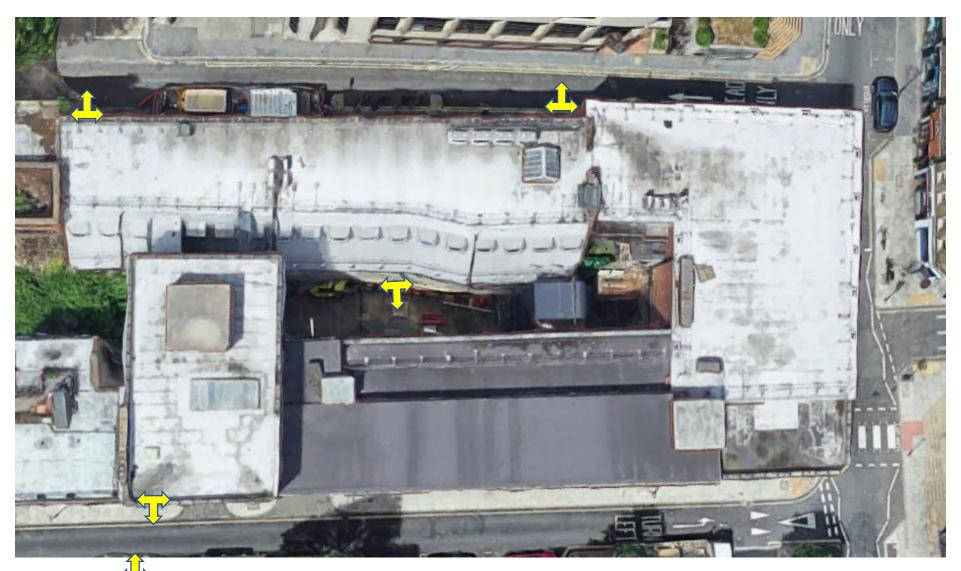
Suggested siting points for Guardian 2 stations with Noise, dust and vibration sensors (110v powered)
