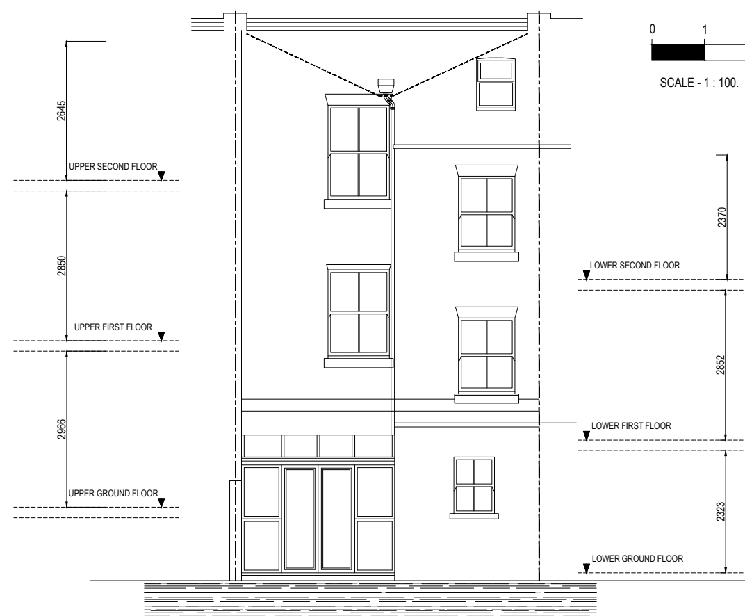
EXISTING REAR ELEVATION
