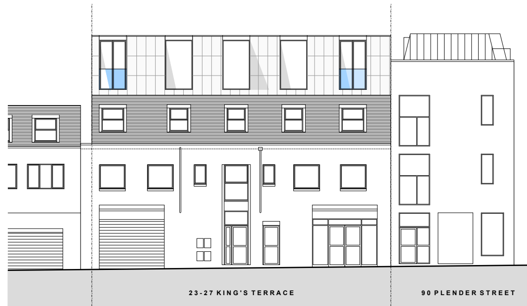
2 SK-003 PROPOSED EAST ELEVATION SCALE@A1 1:100 SCALE@A3 1:200
