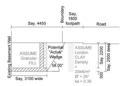
By Inspection, the lateral movements/vertical settlements from an adequately designed/supported temporary excavation and/or permanent structure should not be significant beyond the site boundary, provided that the works are performed in an adequately controlled
