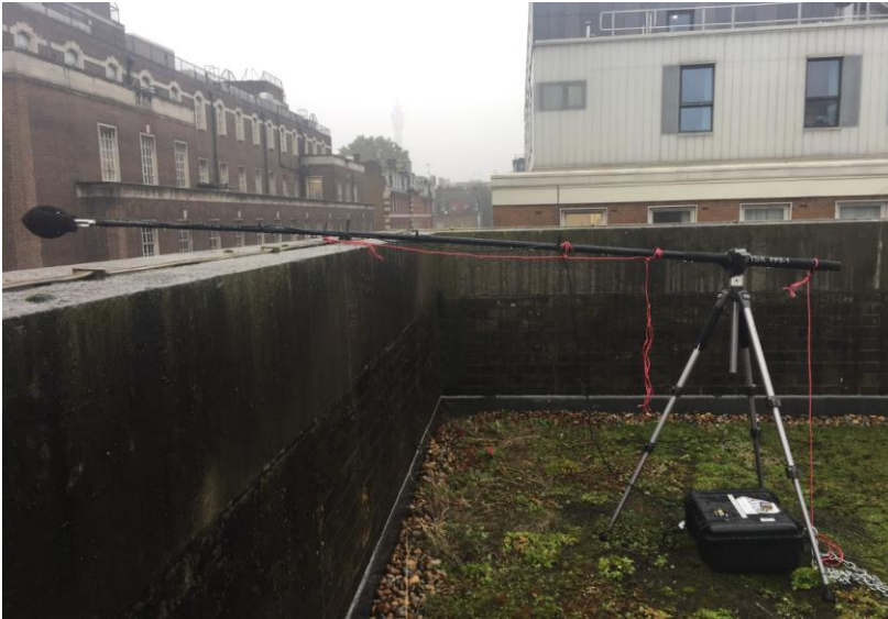
Figure 2: Noise logger set-up, overlooking Bidborough St
