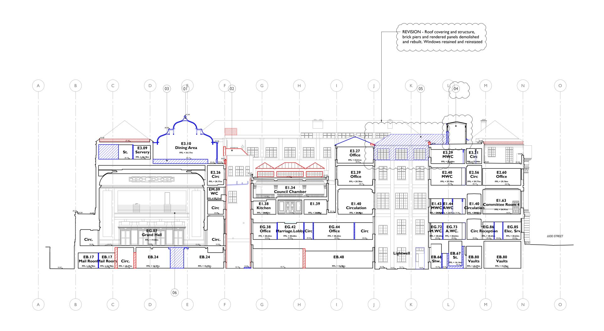
**SECTION F-F PROPOSED DEMOLITIONS AND STRIP OUT** 91205 1:200 @ AI
