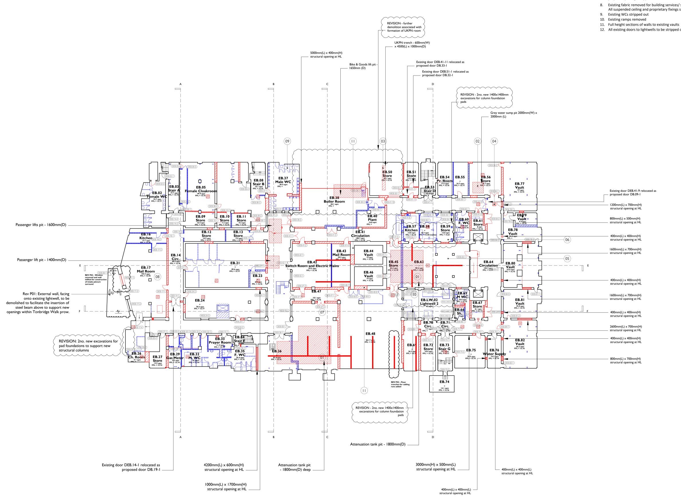
**BASEMENT FLOOR LEVEL PLAN PROPOSED DEMOLITIONS AND STRIP OUT** 91000 I:200 @ AI
