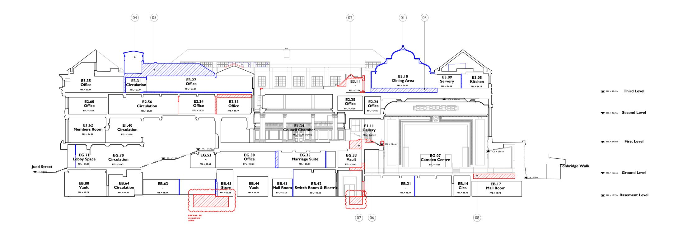
**SECTION E-E PROPOSED DEMOLITIONS AND STRIP OUT** 91204 I:200 @ AI
