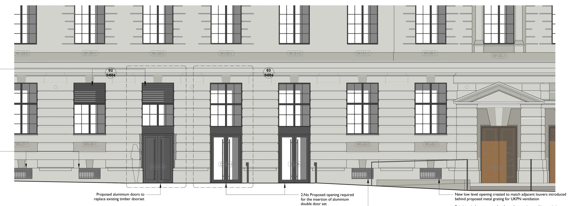
Existing windows removed and new louvers inserted into existing openings for UKPN ventilation. Existing metal grilles in front of opening retained
