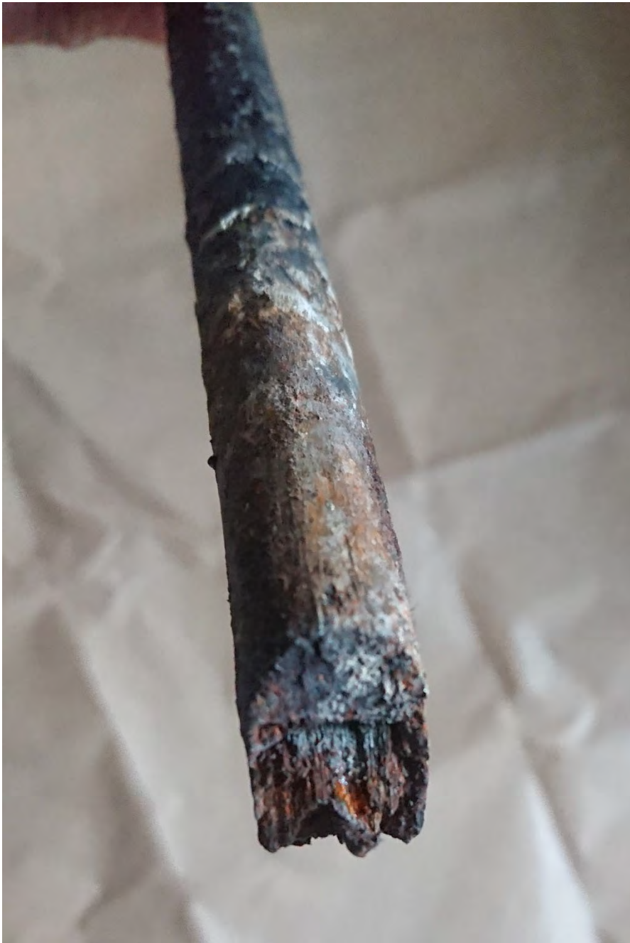
Grain-like appearance of cut end suggests the bars are wrought iron
