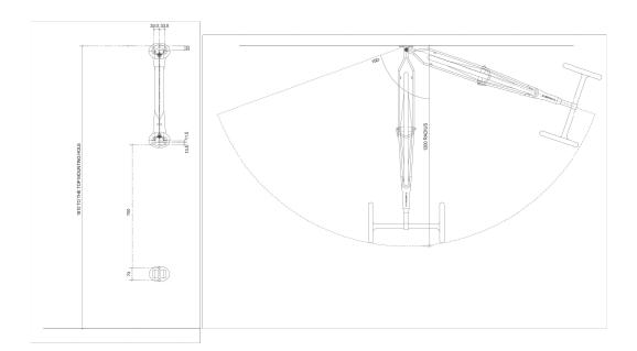
These diagrams are provided as guide only. Bike manufacturers constantly vary the dimensions of their bikes so it is recommended to check before finalising the exact mounting heights.
