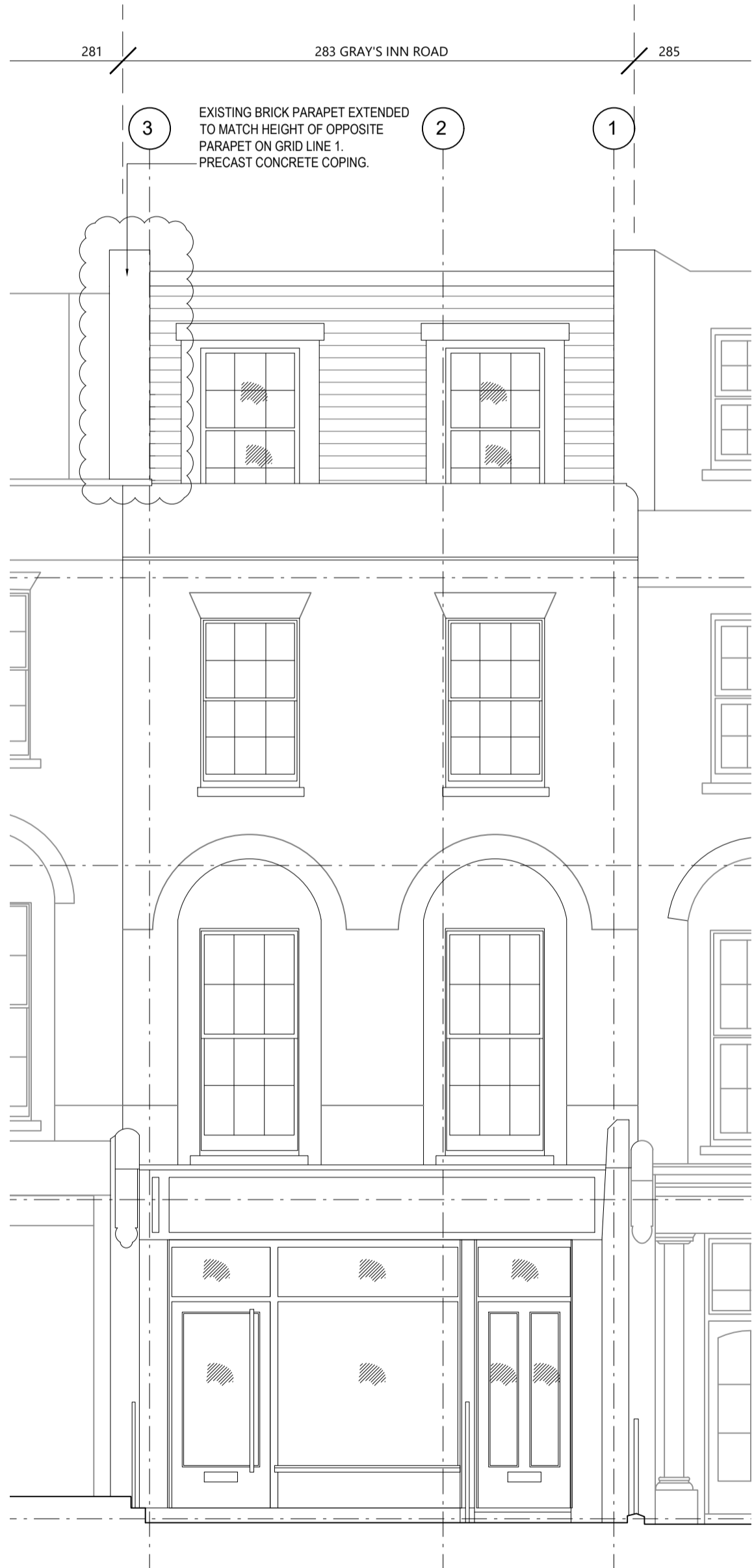
SCALE 1:50@A1 PROPOSED FRONT ELEVATION
