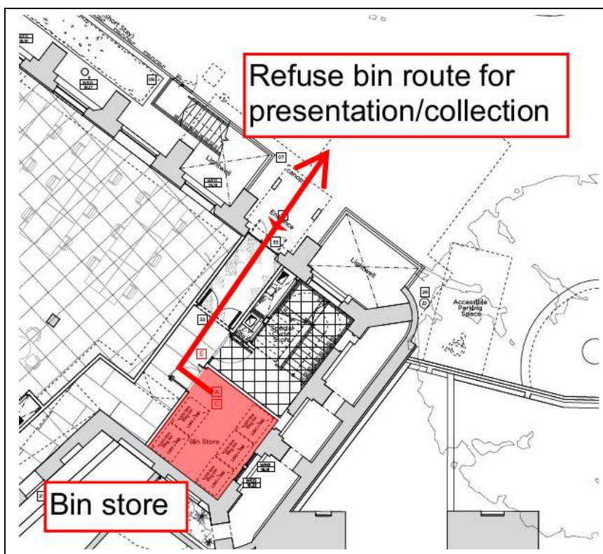
Figure 7.2: The Diorama Waste Store layout – Three-day storage
