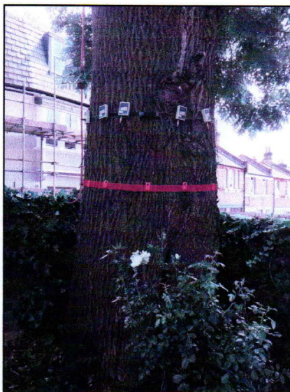
Figure 6: Image Showing PiCUS Test Plane on the north-western Aspect of the Common Ash at 1.3m
