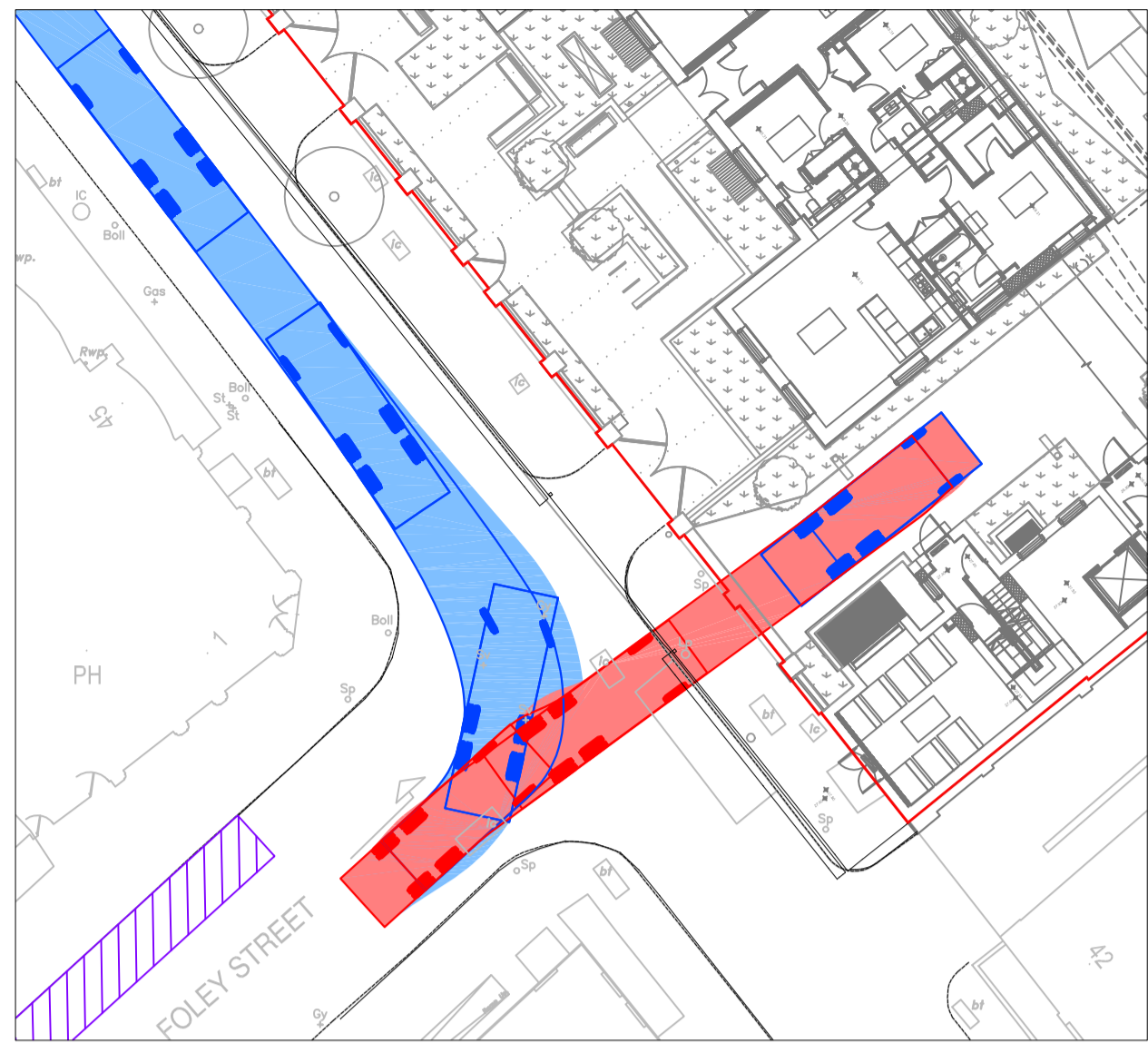
INSET 1 - EXIT MANOEUVRE (Scale 1:250)
