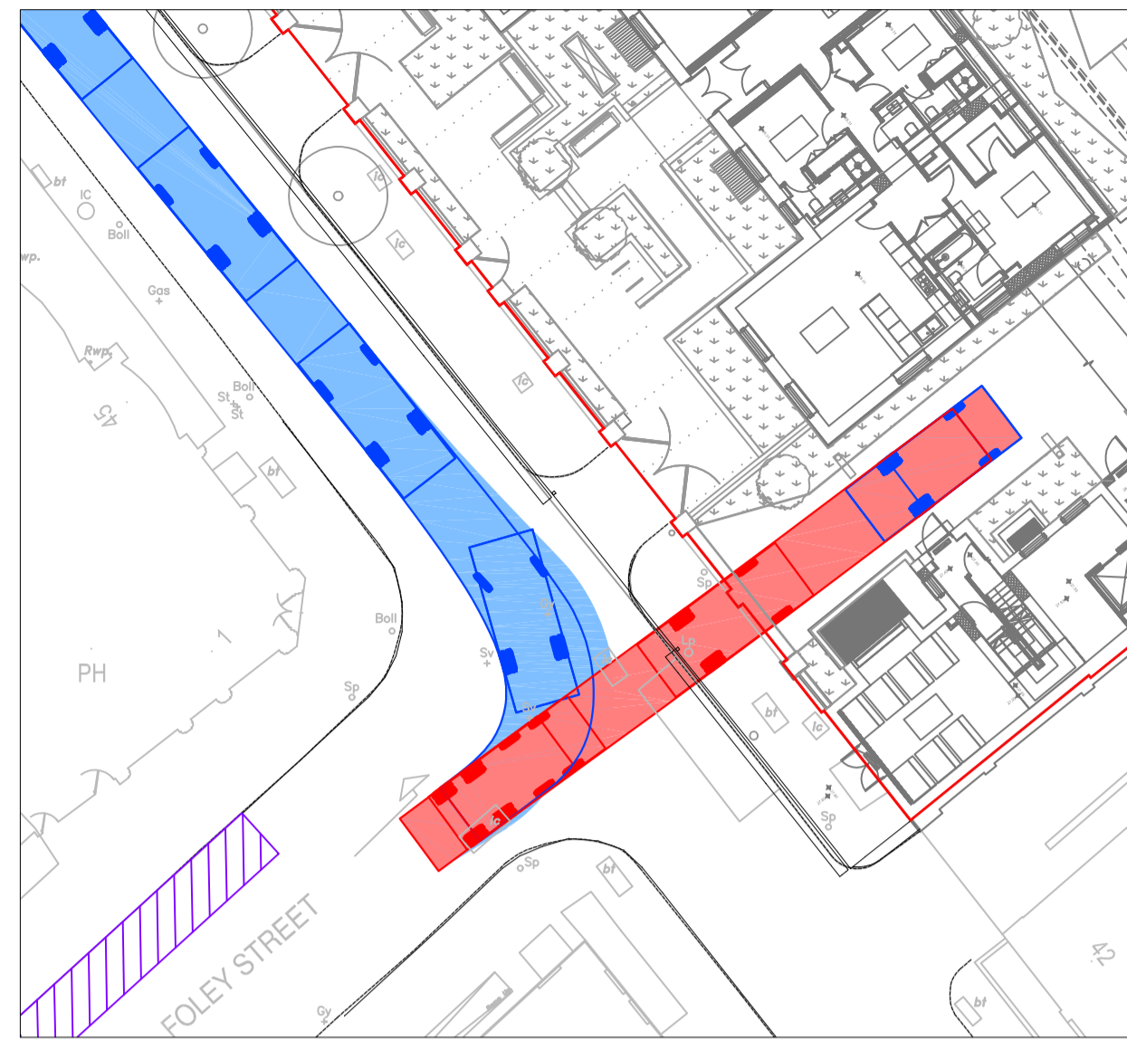
INSET 2 - EXIT MANOEUVRE (Scale 1:250)
