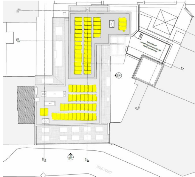
Image shows the propose locations for the PV panels at 8 th floor
