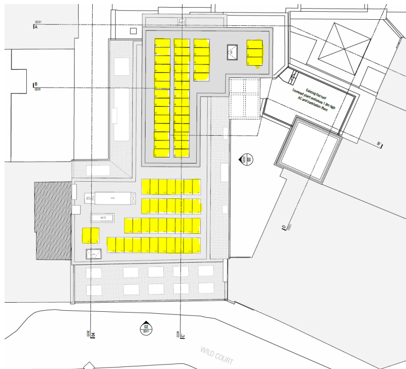
Image above indicates the proposed location for the new PV panels at 8th floor.
