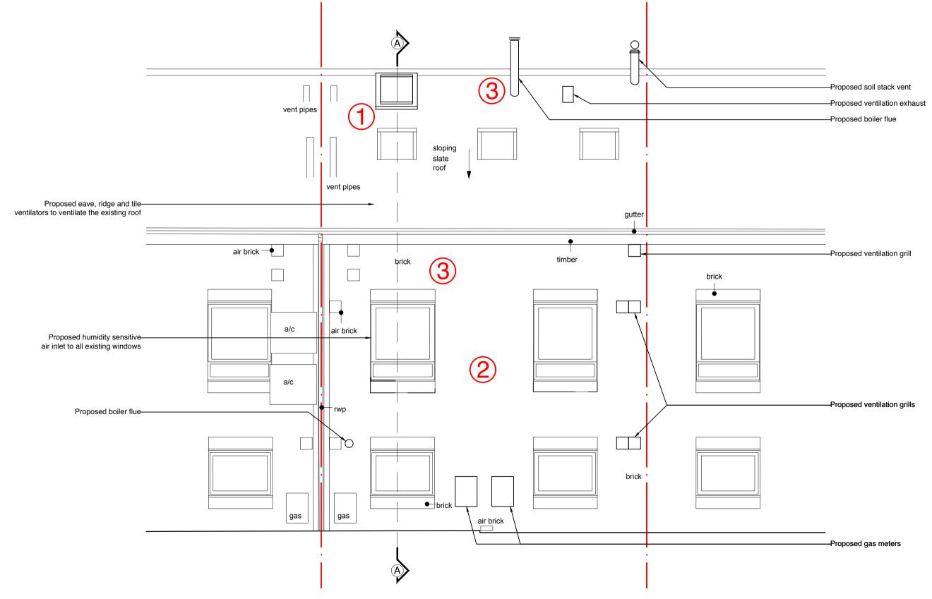
PROPOSED REAR ELEVATION SCALE: 1:100 @ A3
