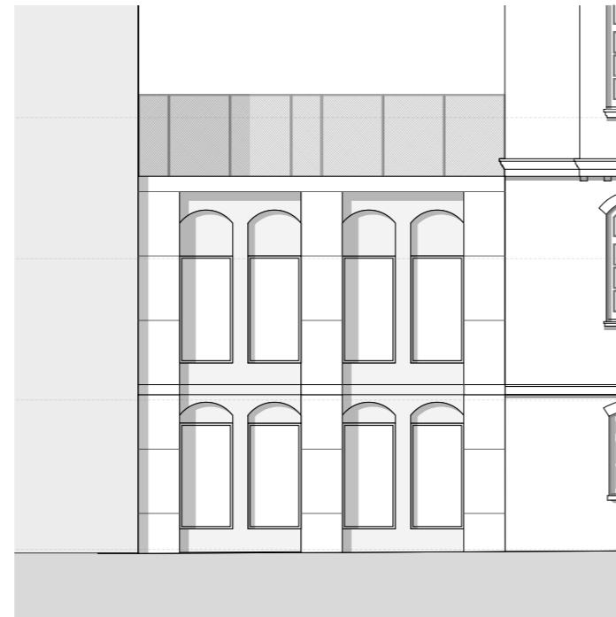
02 Introduction of arched openings works well with existing building but the facade appears overly vertical and too formal.
