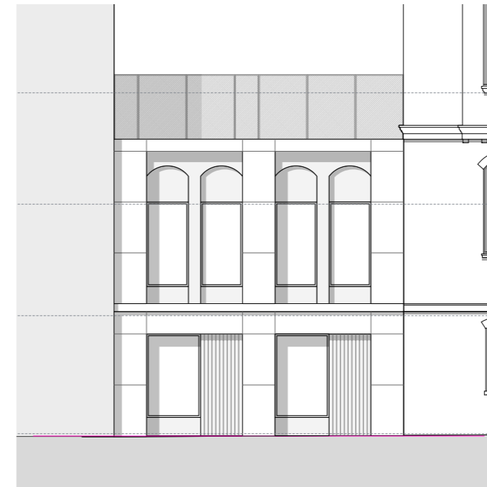
03 Introduction of string course is an improvement, but ground floor lintels too heavy compared to horizontals on the existing building.
