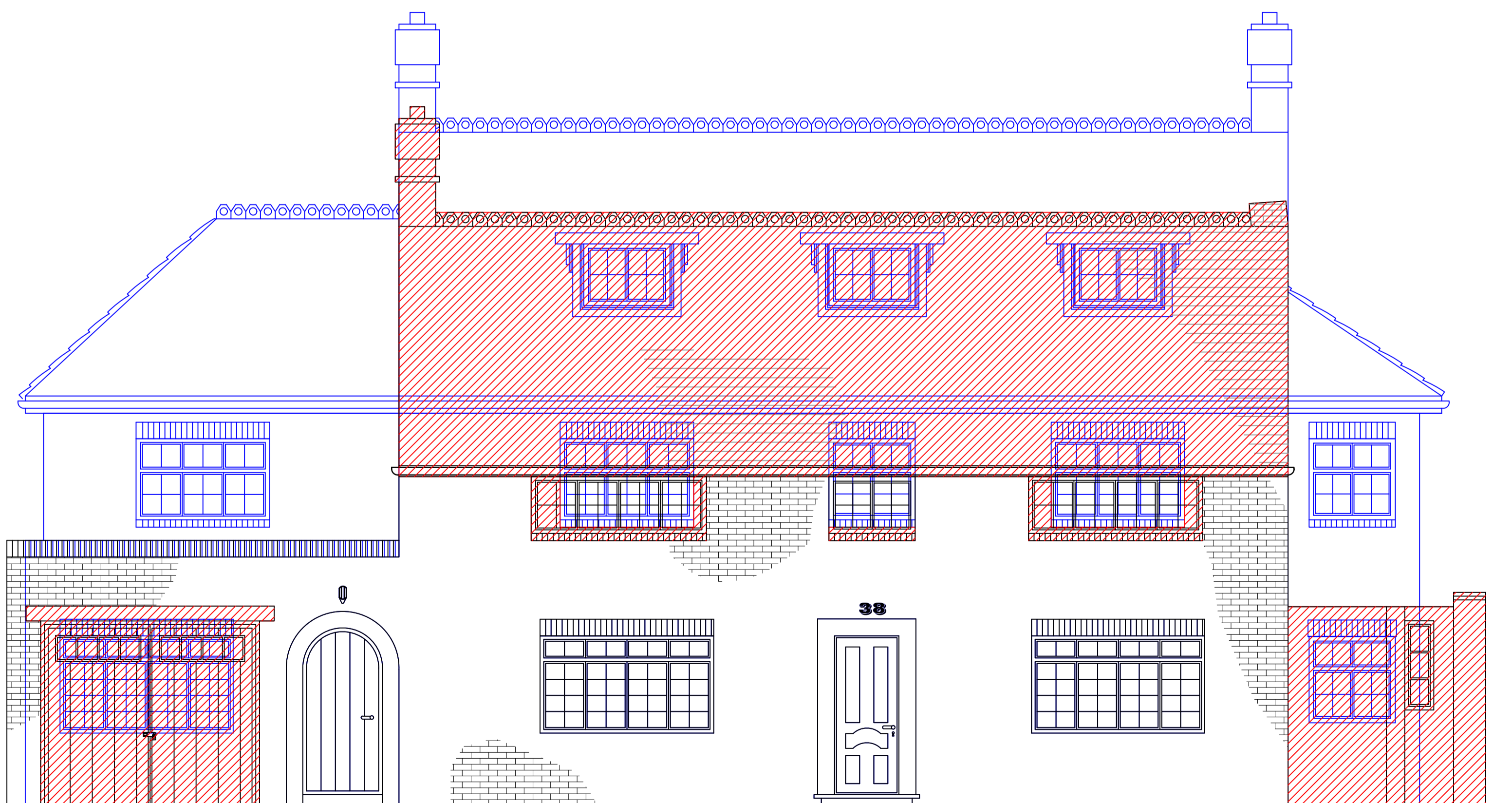
FRONT ELEVATION TOTAL DEMOLITION AREA = 61.4 m 2
