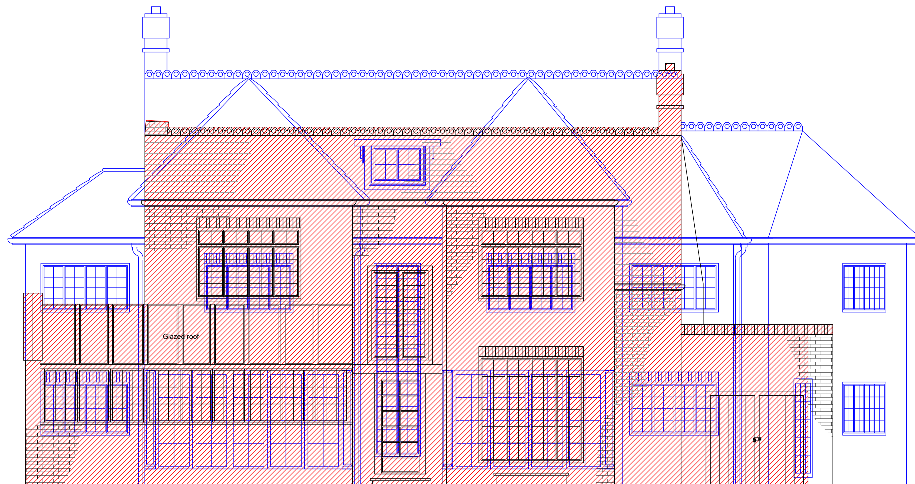
REAR ELEVATION TOTAL DEMOLITION AREA = 119.5 m 2
