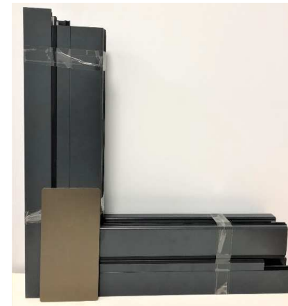
Schueco ASS-80FD Samples (Incorrect finish)
