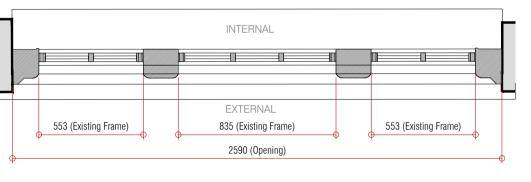
Existing Window:WG-09 Ground Floor Plan
