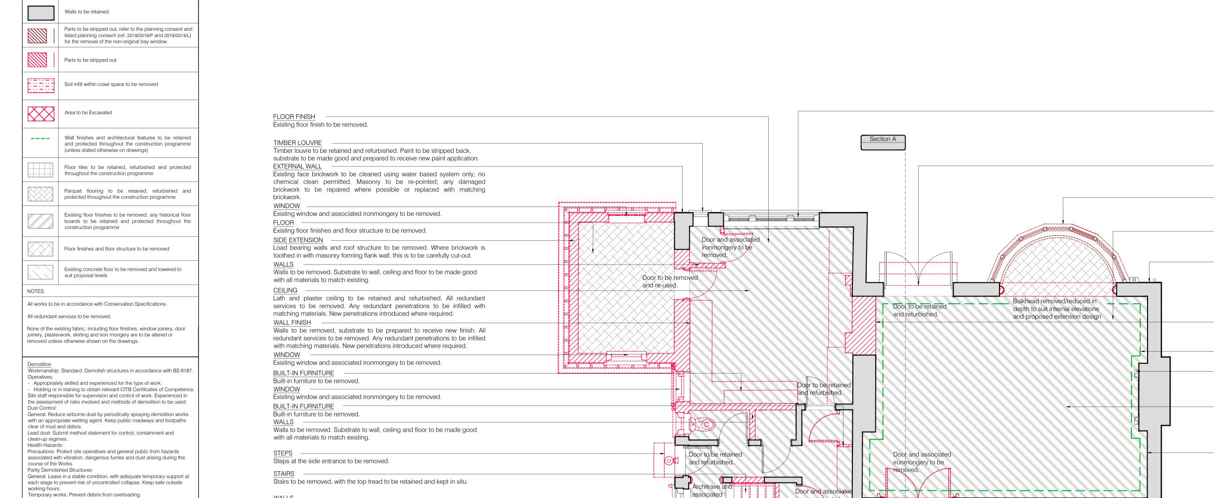
Walls to be removed. Substrate to wall, ceiling and floor to be made good
