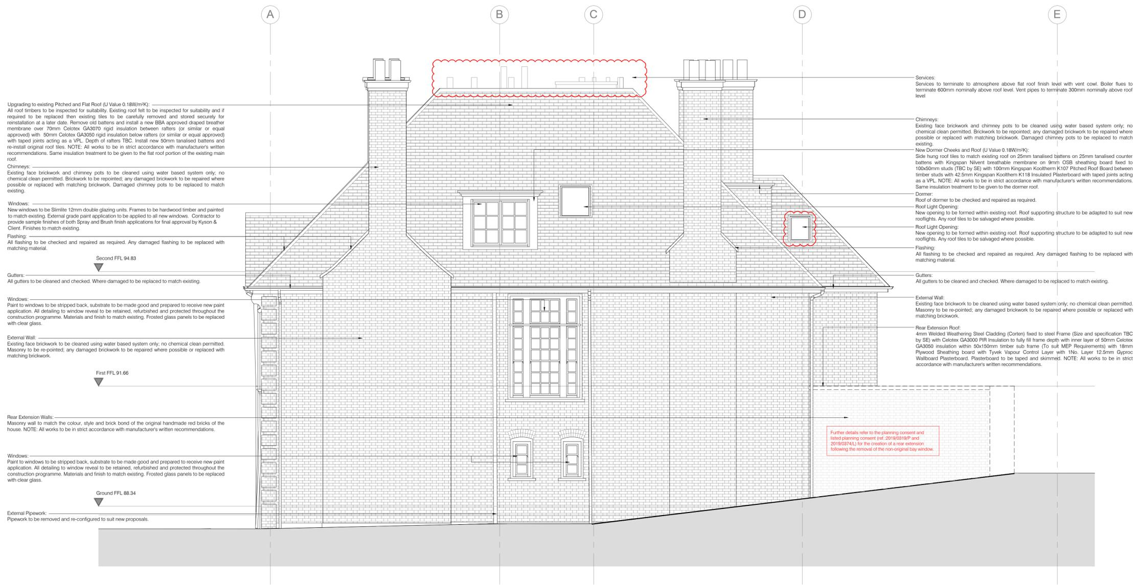
**Upgrading to existing Pitched and Flat Roof (U Value 0.18W/m<sup>2</sup>K):**
